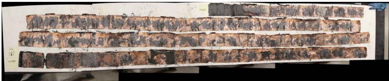
**Figure 12.** Cell 6 electrode unwound on table.
