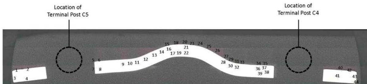
**Figure 9.** Microhardness indentation locations of C4–C5 bus bar.
