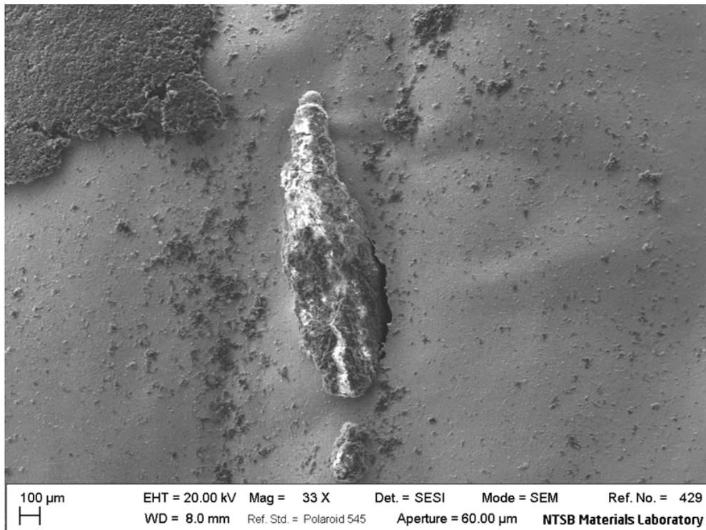
**Figure 15.** Aluminum lump projecting through the bottom of a copper foil wrap, cell 6.
