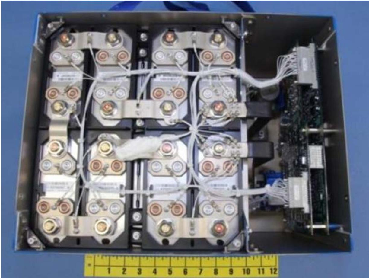
**Figure 1.** Exemplar for the 787 main and APU batteries.
