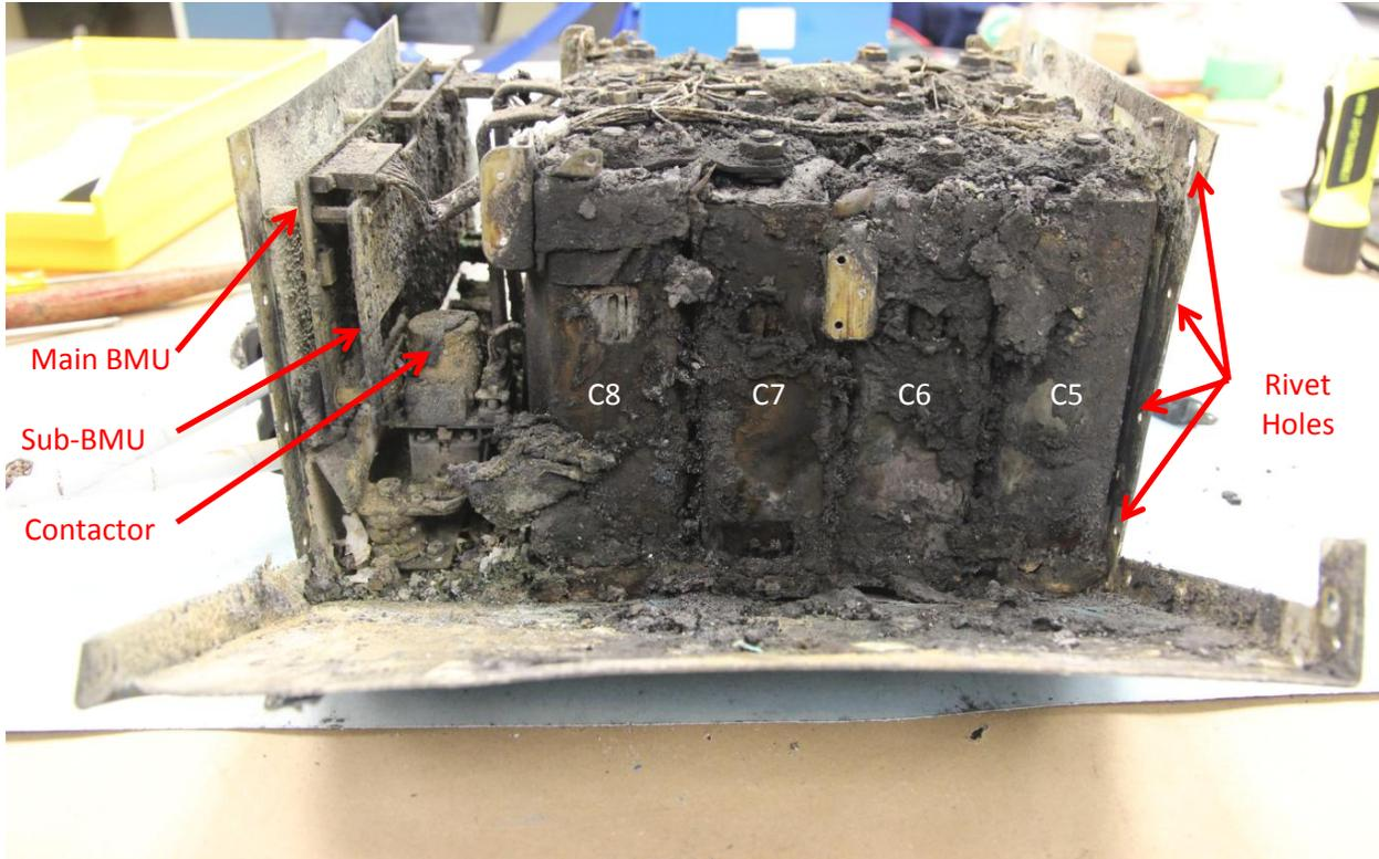
**Figure 6.** View of battery with battery case panel pulled back to reveal cells 5 through 8.
