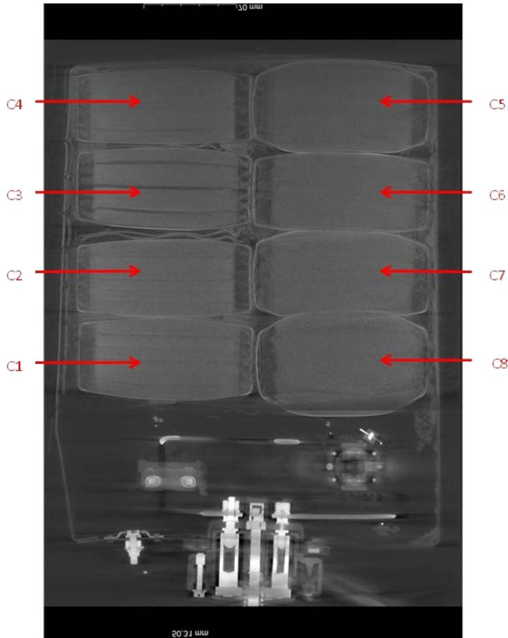
**Figure 5.** Radiographic image of JAL APU battery indicating cell locations.
