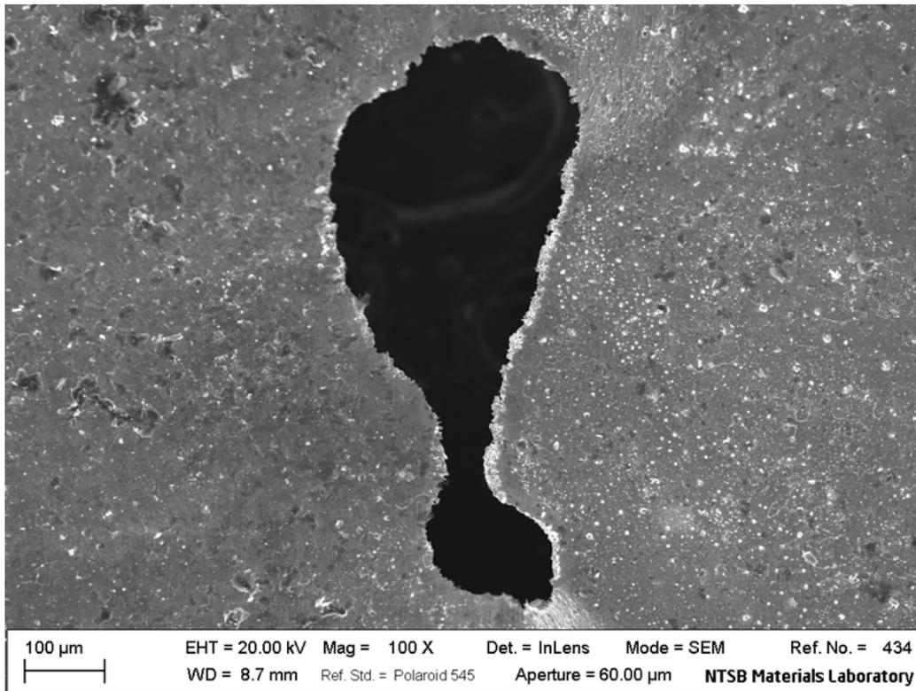
**Figure 16.** Hole in the bottom of the copper foil adjacent to the aluminum protrusion in figure 15, cell 6.
