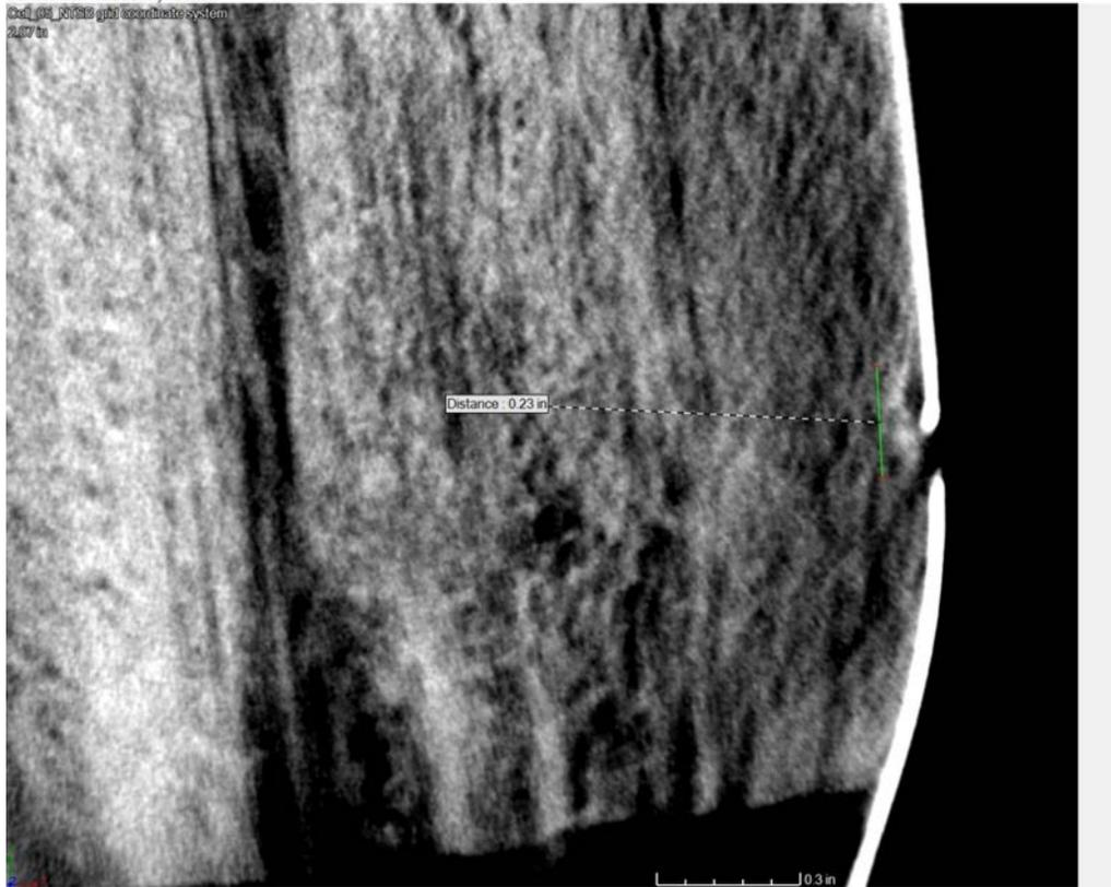
**Figure 11.** CT scan of cell 5 showing breach in case.
