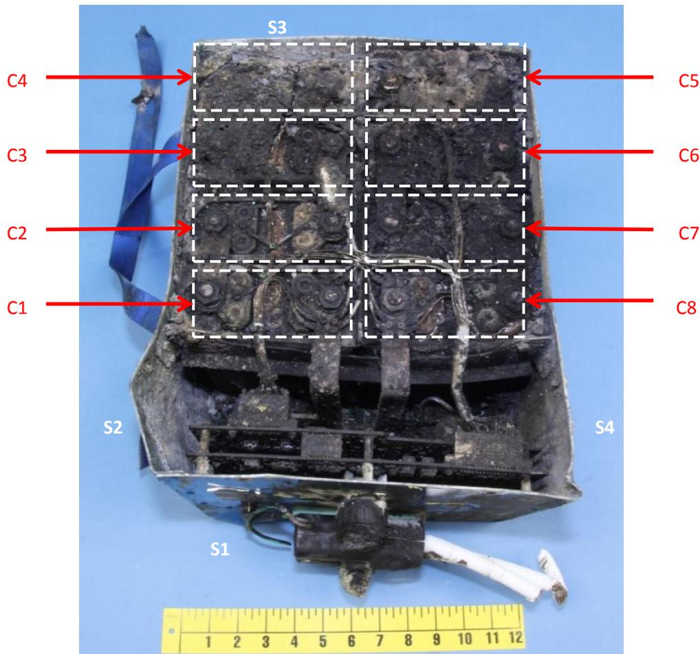
**Figure 4.** Opened battery case showing approximate cell locations.
